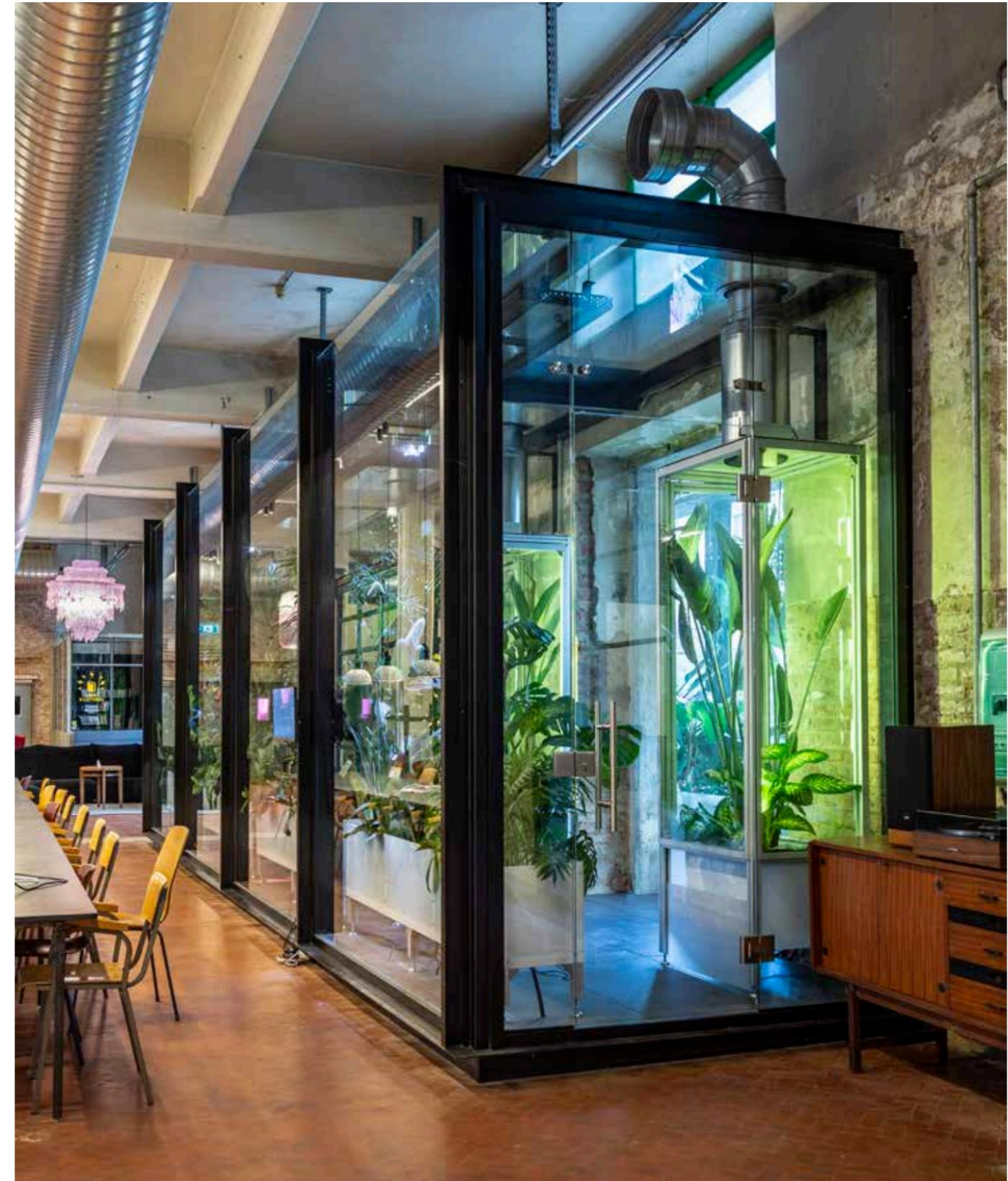
Above. Another glimpse of the first prototype built at the Manifattura Tabacchi in Florence. The Air Factory requires little maintenance, irrigation is automated, and the technical light inside has specific frequencies to promote photosynthesis.
